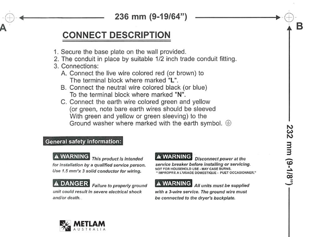
When printing the downloadable Hand Dryer Mounting Template, please ensure the PDF document is printed at Actual Size. If you are unable to print to scale, the use of the measurements on the installation template is paramount. Metlam Australia does not take responsibility for the incorrect print out of mounting templates which result in inaccurate mounting holes being drilled during Hand Dryer installation.
